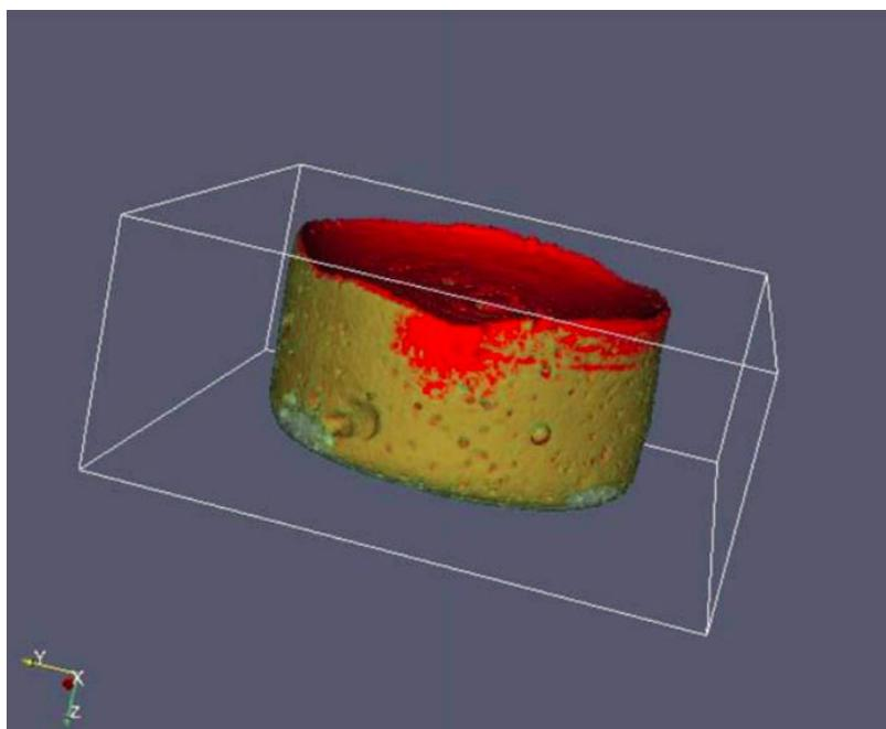
Figure 10. 3D superimposed image of the bonded composite filling restoration before (semitransparent green) and after (red) light-curing (80)
