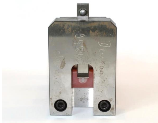
Figure 1a. Setup for the shear bond test according to DIN 13990. The specimen is mounted to a shear guillotine.
