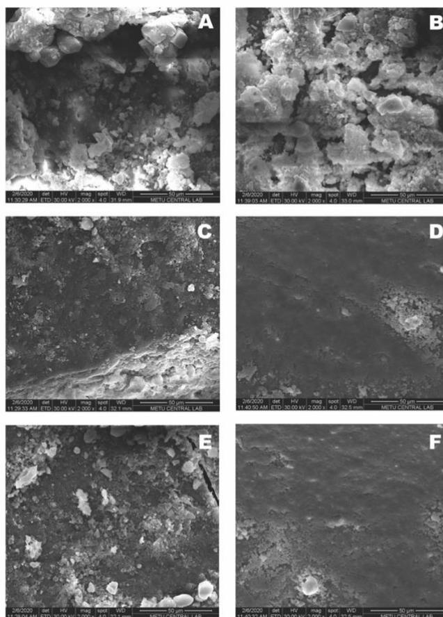
**Fig 1.** Scanning electron micrographs of detect remaining calcium hydroxide: A- PTU F5 ( 2000 X Magnification); B- R50 ( 2000 X Magnification); C- PTU F5-CB ( 2000 X Magnification); D- PTU F5-EDDY ( 2000 X Magnification); E- R50- CB ( 2000 X Magnification); F- R50- EDDY ( 2000 X Magnification).
