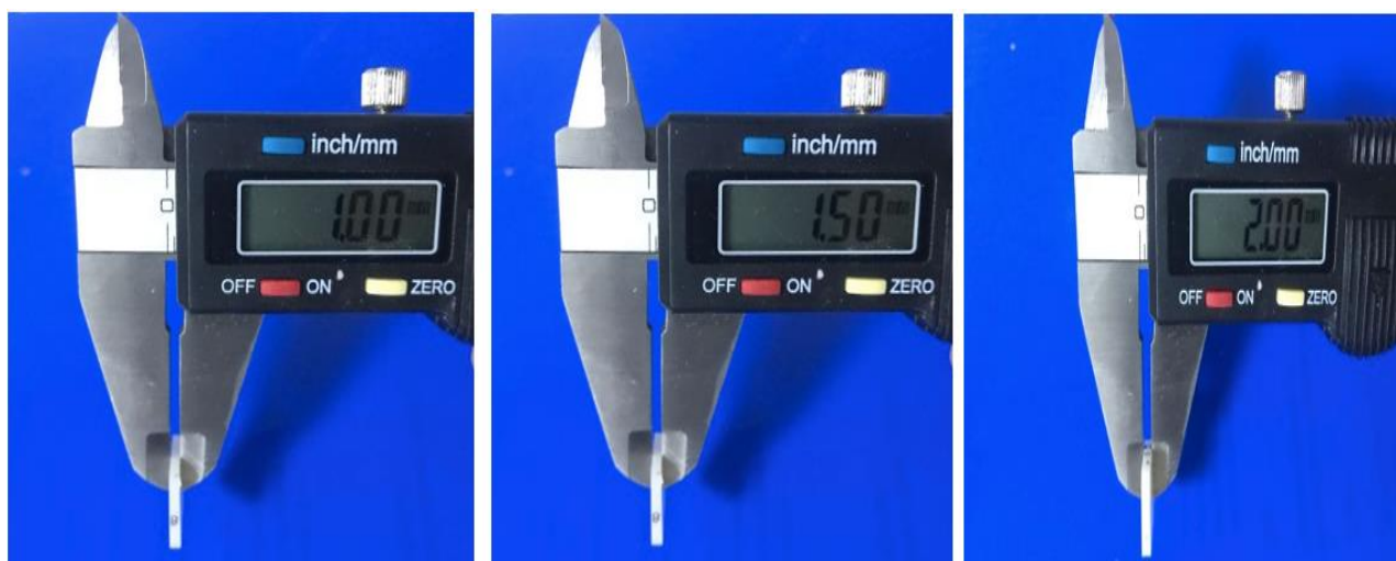
Figure 1. Measurement of the material thickness with a digital caliper.
