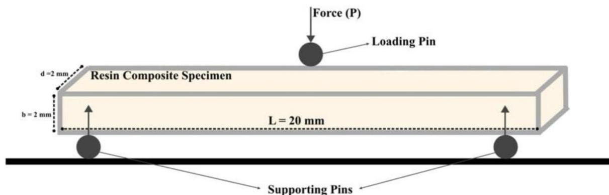
Figure 2. Flexural Strength Application
