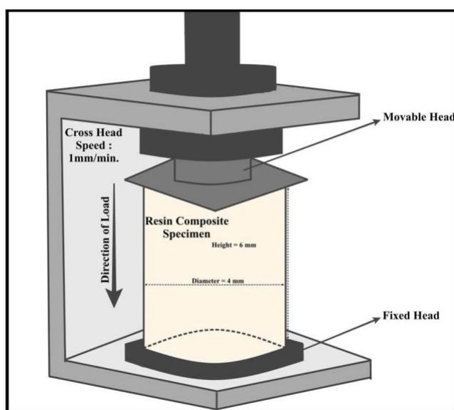
Figure 1. Compressive Strength Application
