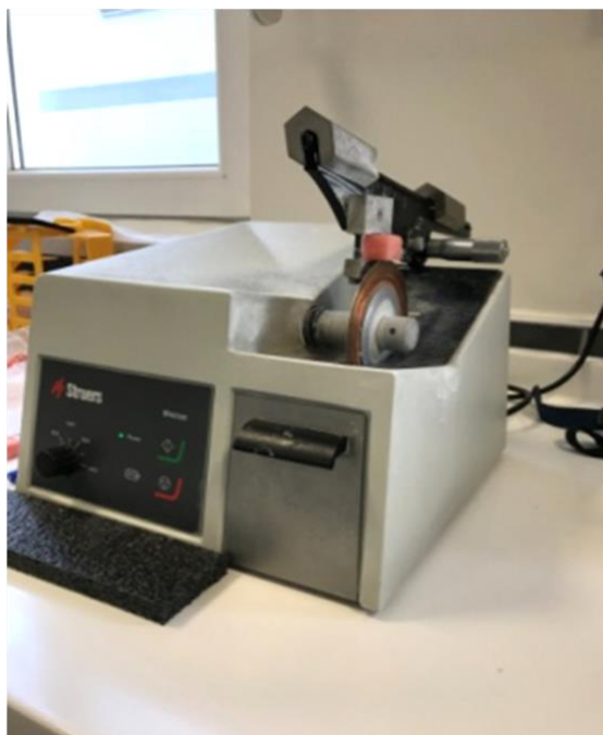
Figure 1. Obtaining cross-sections from teeth embedded in an acrylic block with a precision cutting device.
