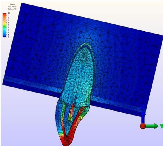
**Figure 3b.** Titanium post model with thermal load (65 °C)
