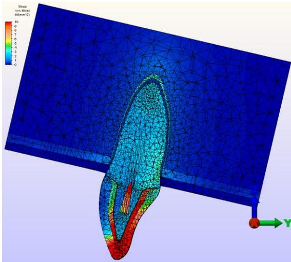
**Figure 2b.** Carbon post model with thermal load (65 °C)
