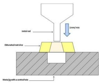
Figure 1. Schematic drawing of the push-out test.
