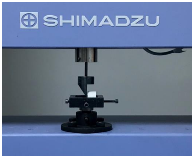
Figure 3. The tip used for the shear test was placed on the glass ceramic sections at an angle of 90°.
